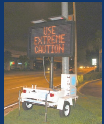
This is a variable message sign used to advise the public of traffic concerns and alert the motorist to watch for pedestrians.
